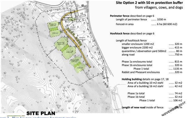
Figure 2 - Plan for new enclosures for target species
