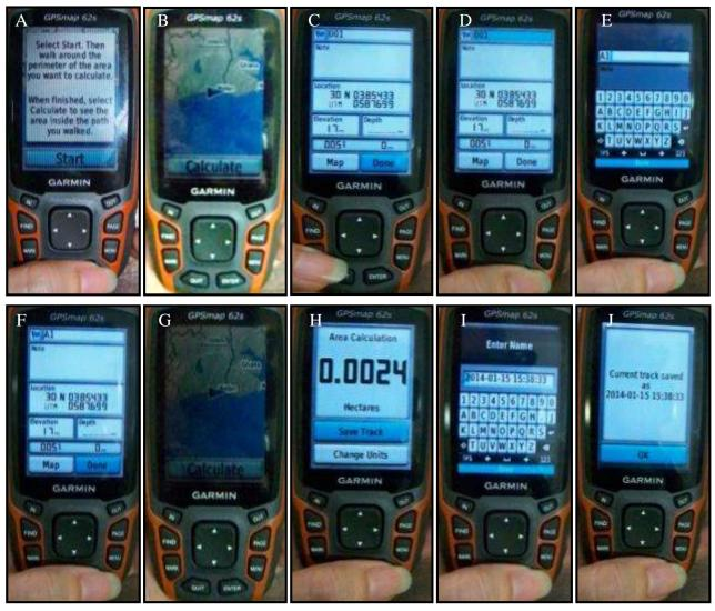
Figure 14: Steps to calculate the area of a land plot with a GPS unit
