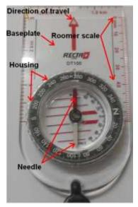
The compass is an essential part of equipment to carry with you in the forest. It can be used along the tracks taken and complements the use of the GPS (Figure 16).
