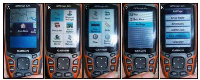
Figure 13: Steps to set up the Area calculation page in the pages menu of a GPS unit
